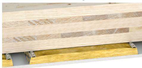
CLT/X-LAM suspended ceiling
