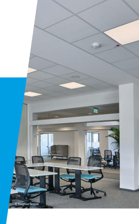
TOPIQ® Alpha 20 is a lightweight and easy-to-install mineral acoustic ceiling tile made of stone wool with a smooth laminated surface appearance
