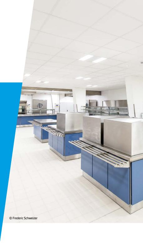
HYGENA TOPIQ® Alpha 20 is a lightweight and easy-to-install mineral acoustic ceiling tile made of stone wool with a smooth laminated surface appearance. The surface is washable and antimicrobial.
