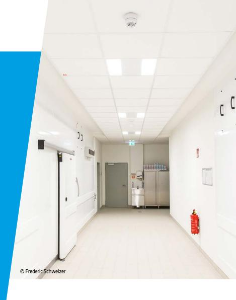
HYGENA TOPIQ® Alpha 15 is a lightweight and easy-to-install mineral acoustic ceiling tile made of stone wool with a smooth laminated surface appearance. The surface is washable and antimicrobial.
